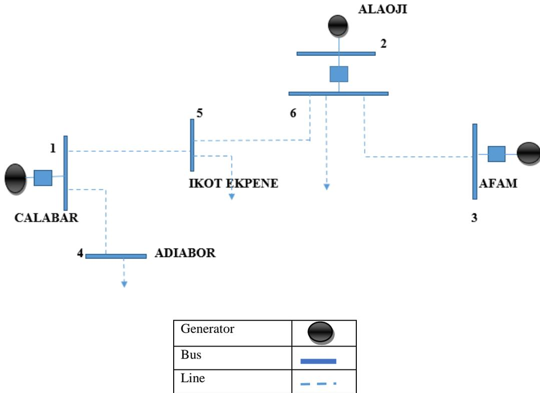
**Figure 1:** Line diagram of Nigeria 330KV sub-network of Calabar, Alaoji and Afam.
