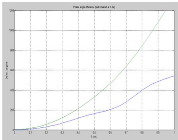
**Figure 9:** Three phase fault on line 6-5 fault clearing time is 0.8-sec system is unstable.
