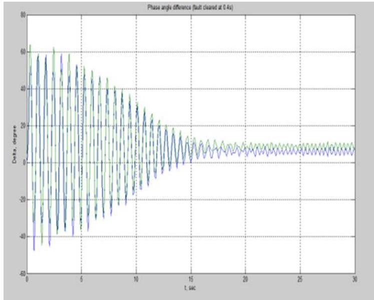
**Figure 8:** Three phase fault on line 6-5 fault clearing time is 0.4-sec system is stable.
