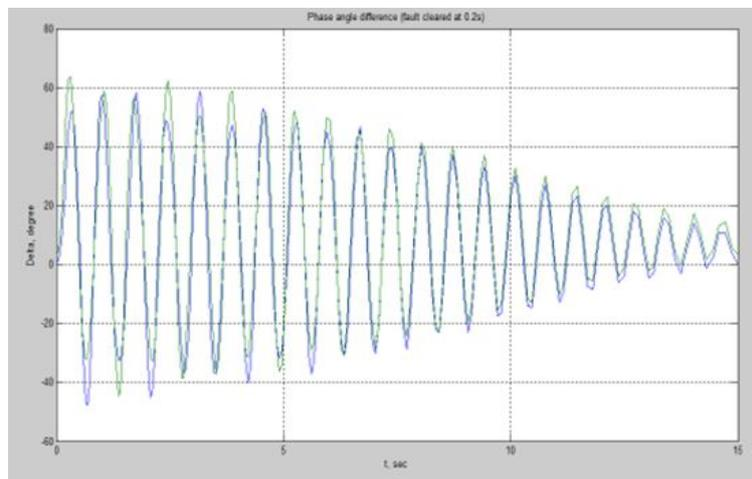
**Figure 4:** Three phase fault on lines 1-5 fault clearing time is 0.2-sec system is stable.
