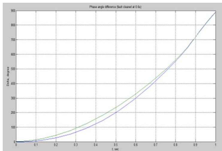
**Figure 5:** Three phase fault on line 1-5 fault clearing time is 0.6-sec system is unstable.
