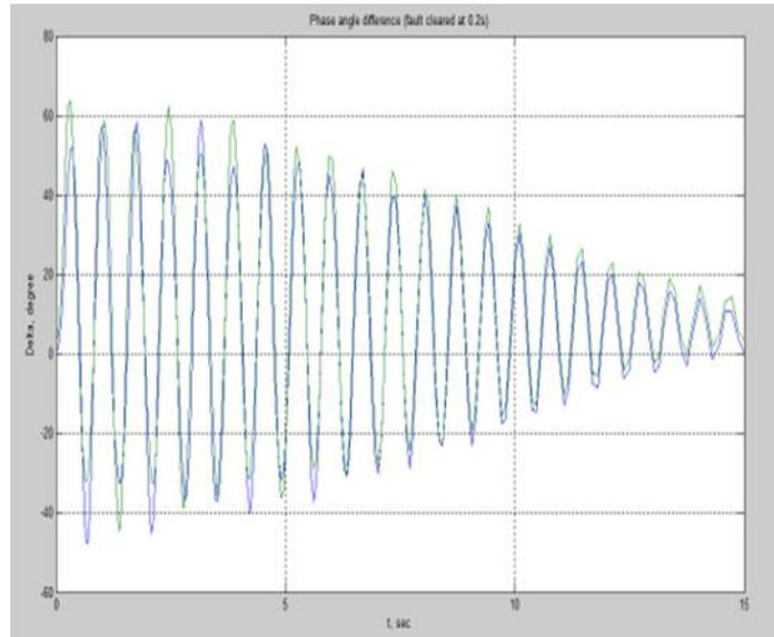
**Figure 6:** Three phase fault on lines 3-6 fault clearing time is 0.3-sec system is stable.
