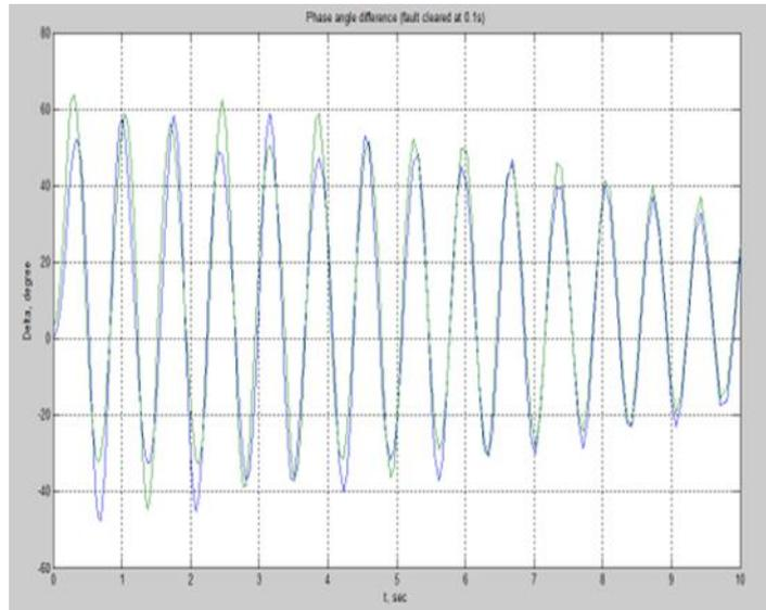
**Figure 2:** Three phase fault on lines 1-4 fault clearing time is 0.1-sec system is stable.
