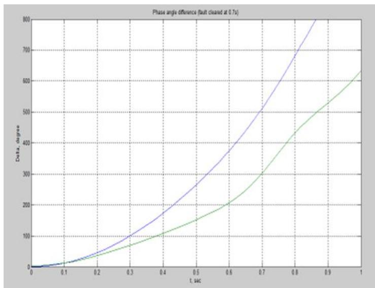
**Figure 7:** Three phase fault on lines 3-6 fault clearing time is 0.7-sec system is unstable.
