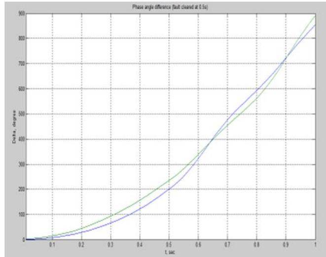
**Figure 3:** Three phase fault on lines 1-4 fault clearing time is 0.5-sec system is unstable.
