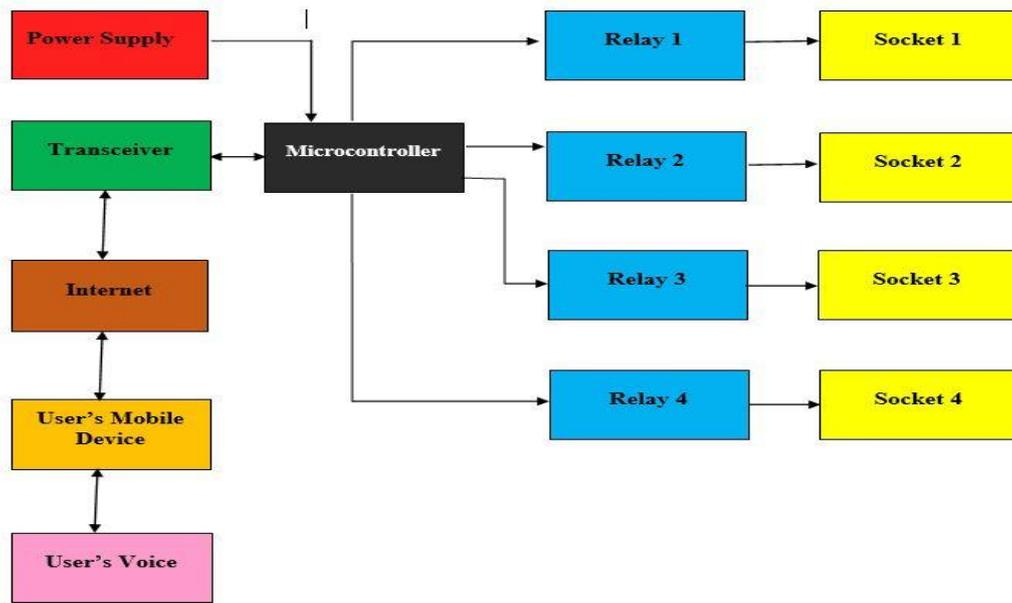
**Figure 1:** block diagram for the proposed design.
