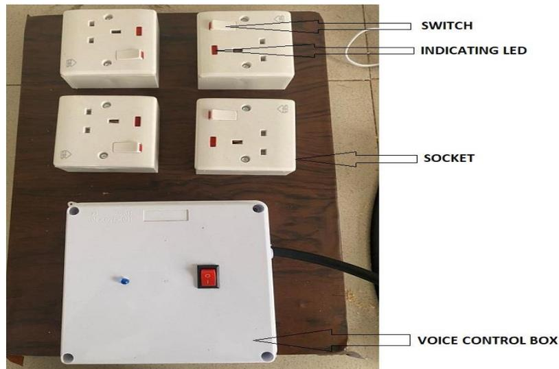
**Figure 6:** Labeled designed artefact.
