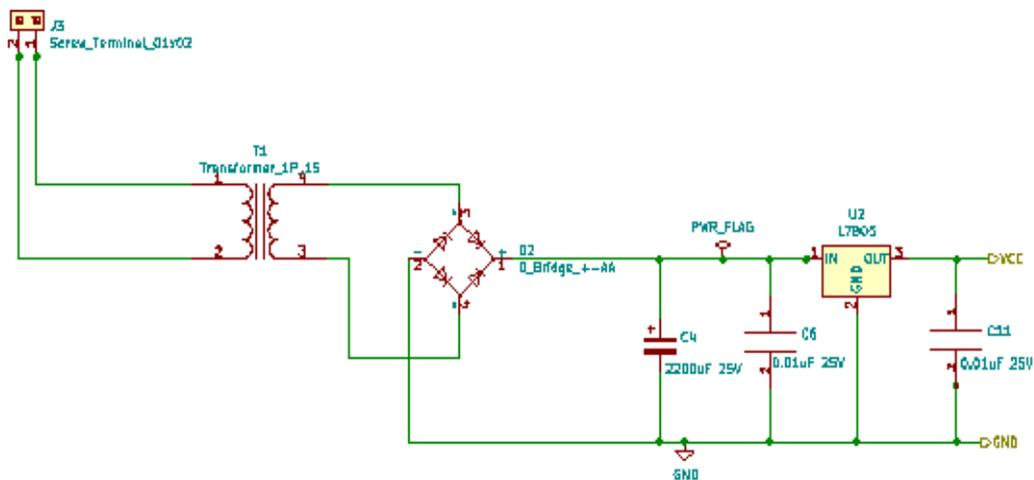
Figure 4: power supply circuit.
