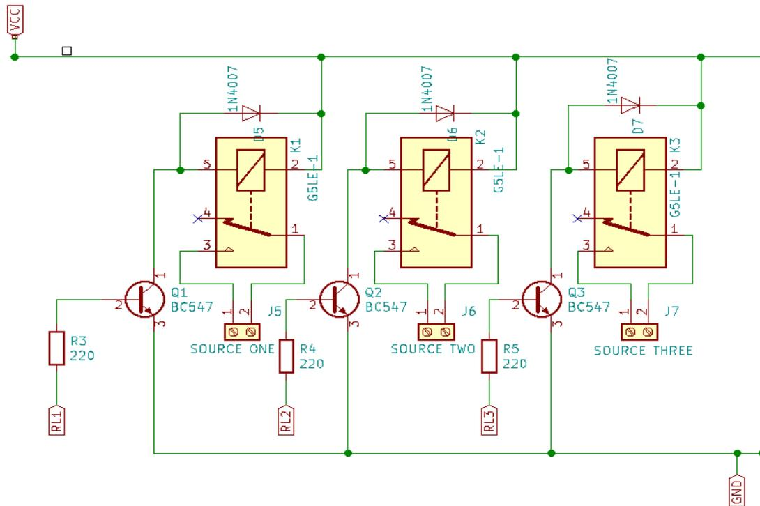
Figure 5: Relay circuit.
