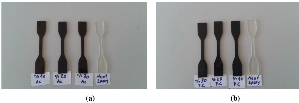
Figure 5: Prepared natural waste filler composites (a) acorn (A.C.) based samples, (b) pine cone (P.C.) based samples
