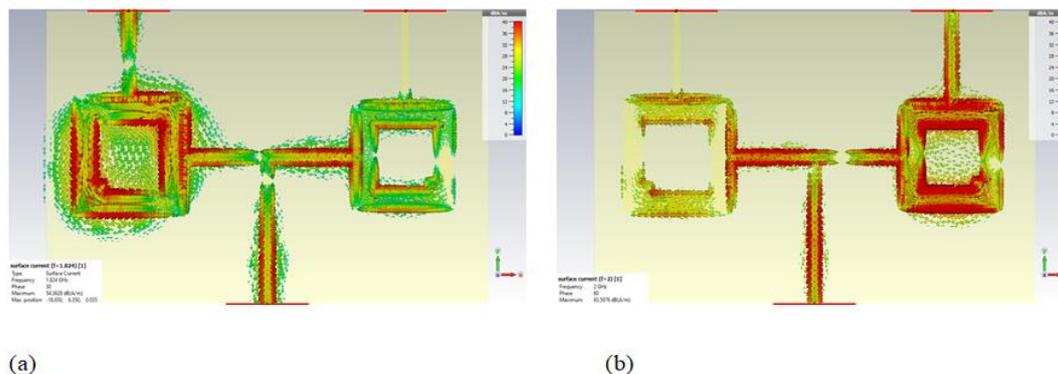
**Figure 5:** Distributions of surface currents of the proposed diplexer (a)  $f_t = 1.82 \text{ GHz}$  and (b)  $f_r = 2 \text{ GHz}$ .
