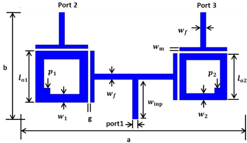
**Figure 3:** The final configuration of the proposed diplexer.
