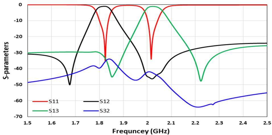
**Figure 4:** Simulated scattering parameters of the proposed diplexer.
