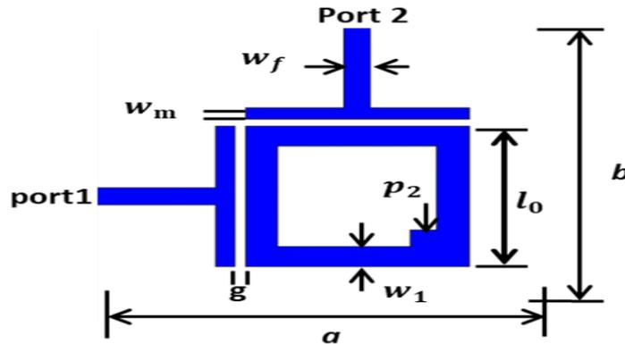
**Figure 1:** The configuration of proposed dual-mode BPF.
