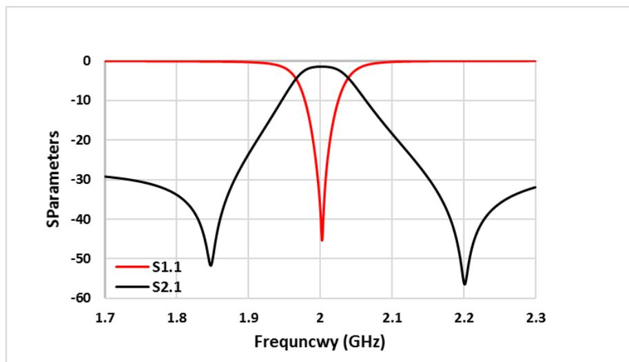
Figure 2: Simulated scattering parameters of the proposed BPF.
