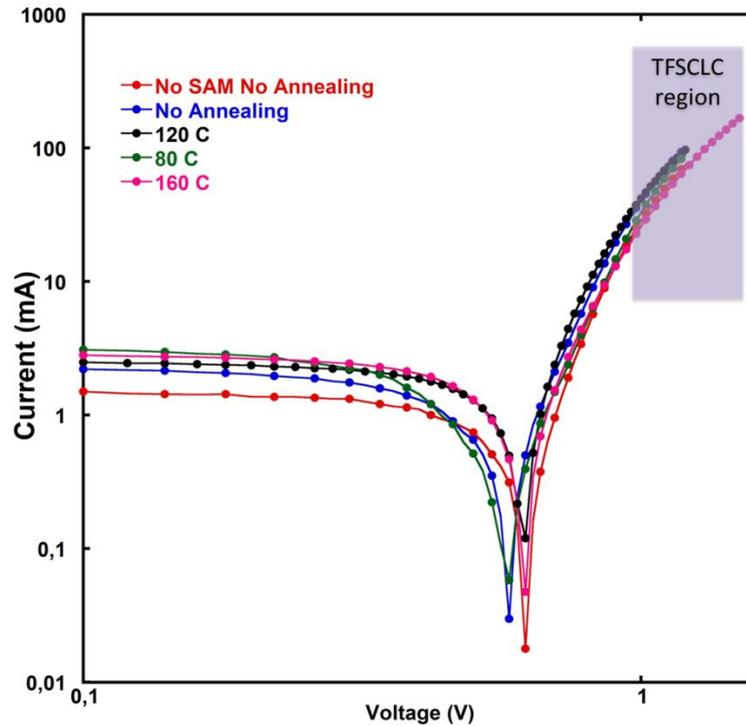
**Figure 2:** The I-V characteristic of P3HT:PCBM based organic solar cell modified with PANPBA self-assembled interlayer.
