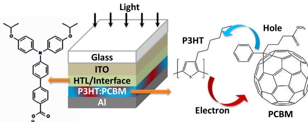
**Figure 1:** Schematic diagram of a donor-acceptor based organic solar cell with conventional architecture and corresponding energy band diagram in eV.
