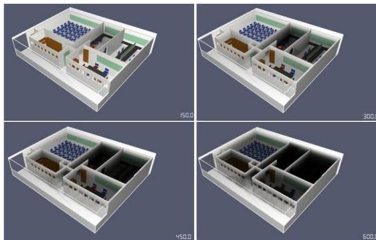
**Figure 5:** Fire simulation in PyroSim.
