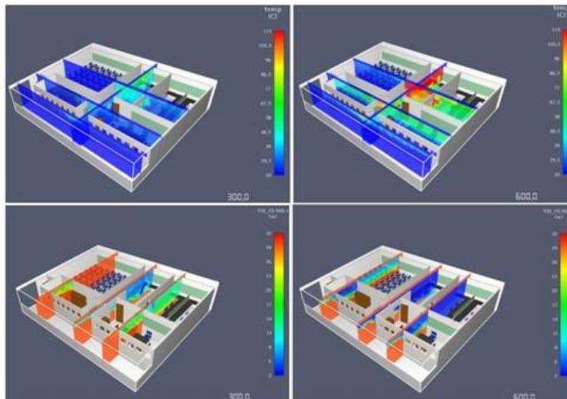
**Figure 4:** Temperature and visibility slices.
