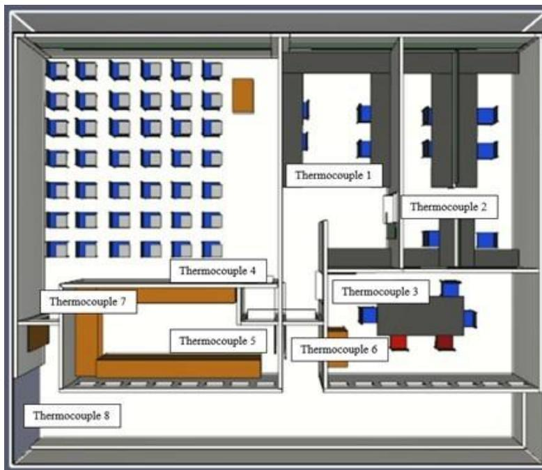
Figure 8: Thermocouple locations.
