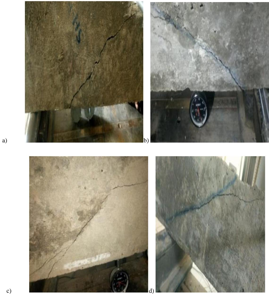
**Figure 23:** Crack pattern of diagonally casted shear beams; a) CSB b) SB-I1/3 c) SB-I1/4 d) SB-I1/5.
