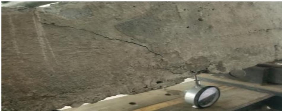
**Figure 12:** mode of Quarter spanned vertical interface shear beam (SB-V1/4).
