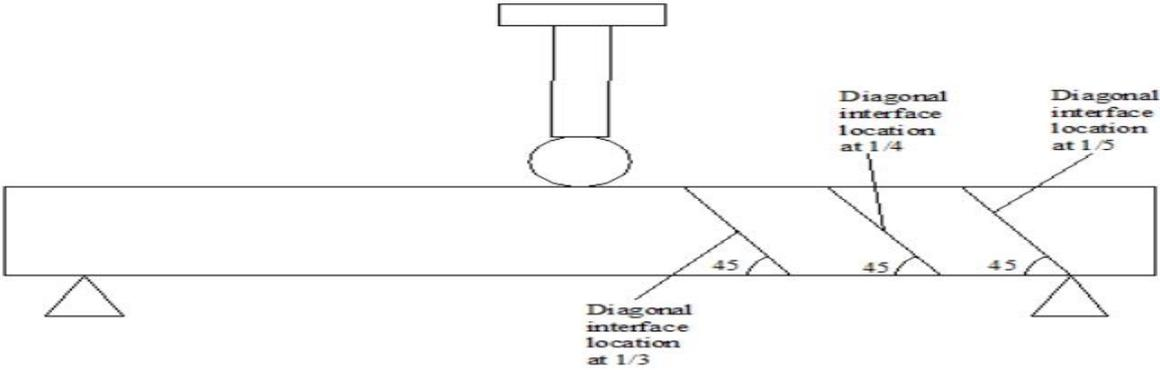
Figure 6: Diagonal interface locations for shear critical beam.
