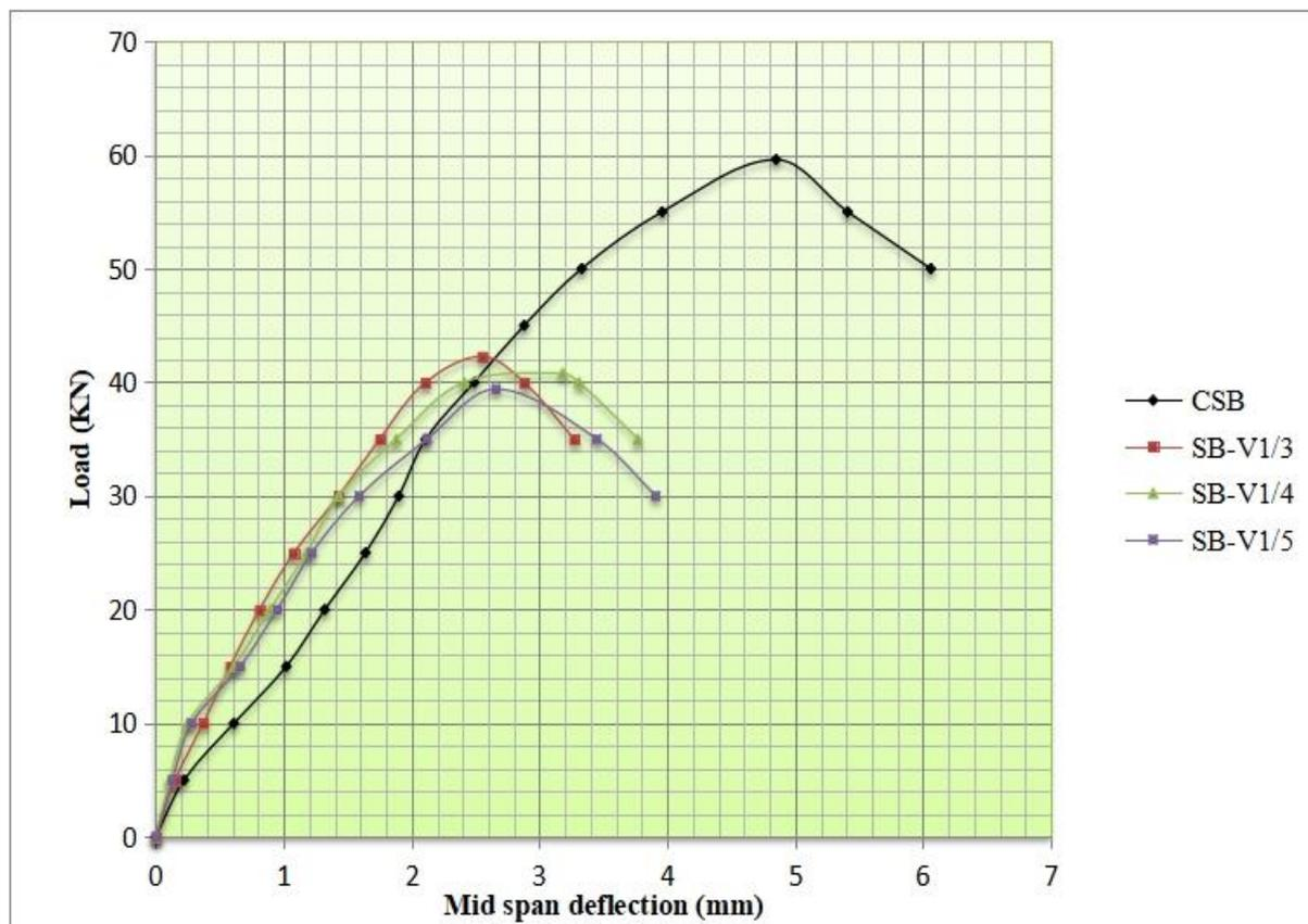
**Figure 14:** Load versus deflection curves for vertically casted shear beams.
