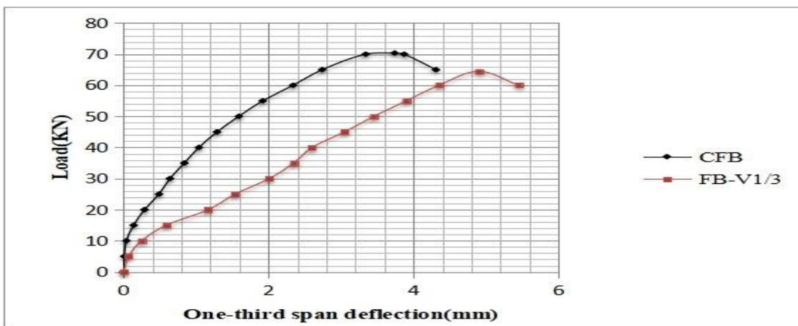
**Figure 22:** Relative load-deflection curves for flexural beams (CFB vs FB-V1/3).
