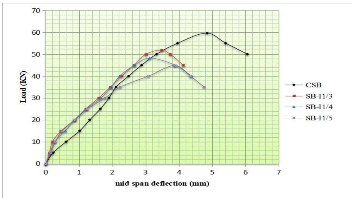
Figure 16: Load versus mid span deflection curves for diagonally casted shear beams
