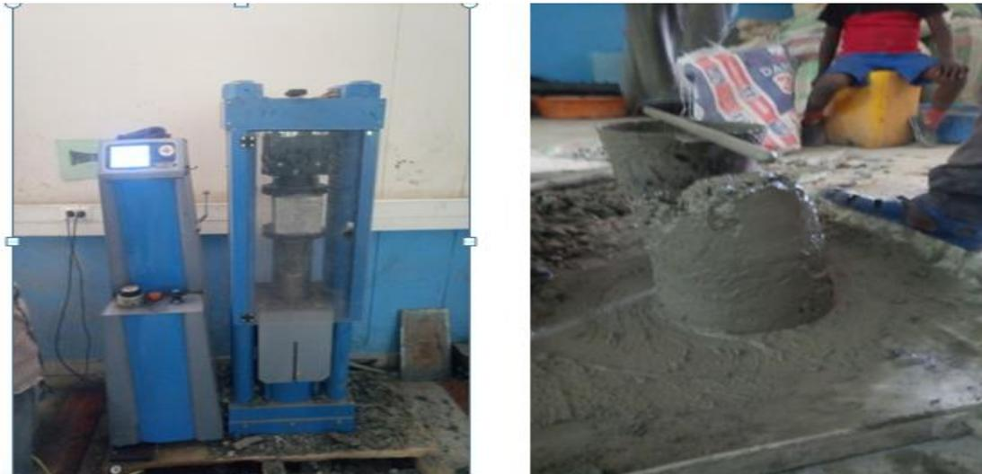
**Figure 8:** Setup of compression test machine and workability (slump test).
