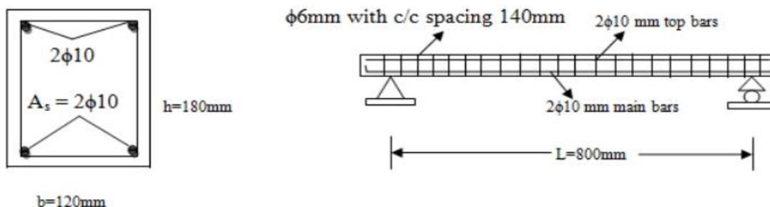
Figure 3: Detail of cross section of the flexural beam specimens.
