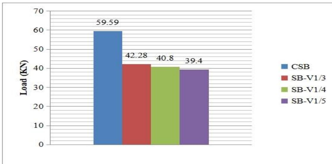
**Figure 15:** Variation of load carrying capacity for vertical interface shear beams.
