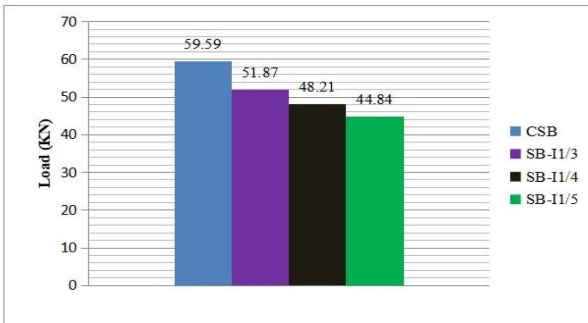
**Figure 17:** Variation of load carrying capacity for diagonal interface shear beams.
