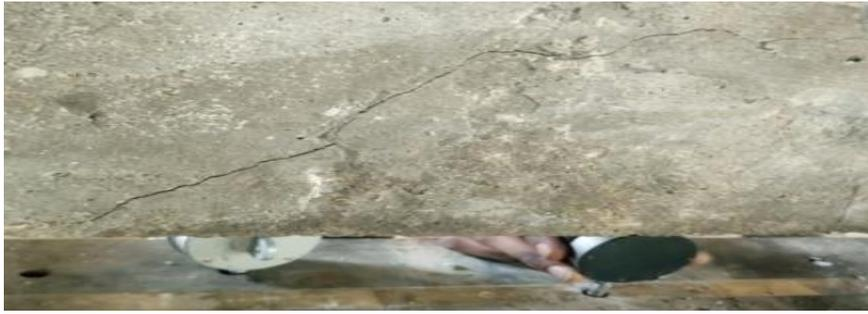
**Figure 11:** mode of One-third spanned vertical interface shear beam (SB-V1/3).
