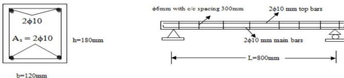
Figure 4: Detail of cross section of the shear beam specimens.
