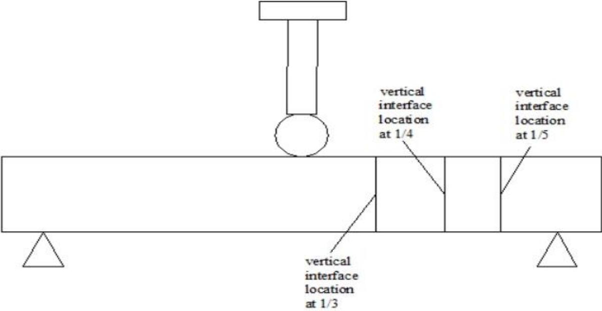
Figure 5: vertical interface locations for shear critical beam.
