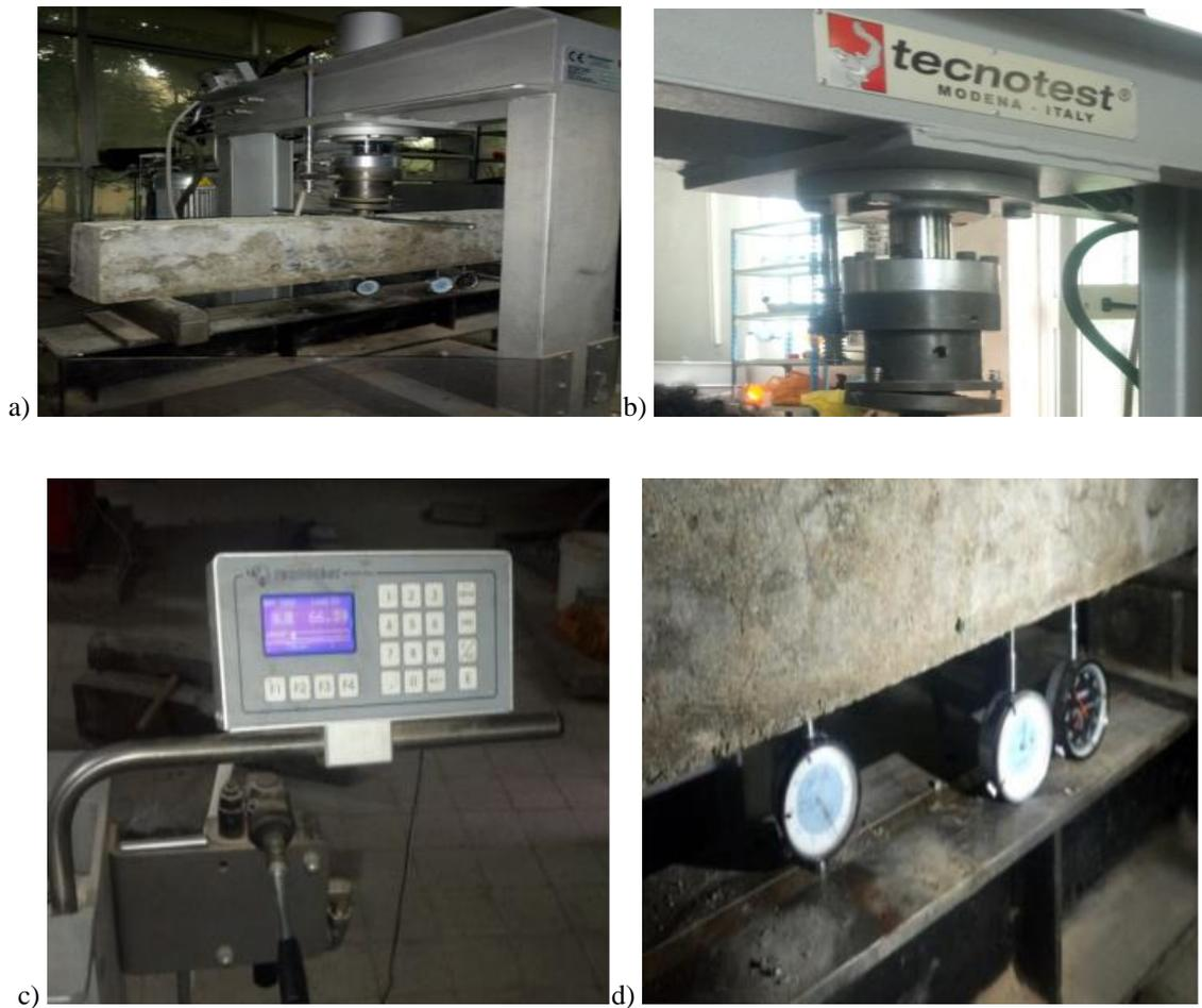
**Figure 10:** Flexural testing machine a) Full setup b) Loading piston c) Digital load reading cell d) Dial Gauges.
