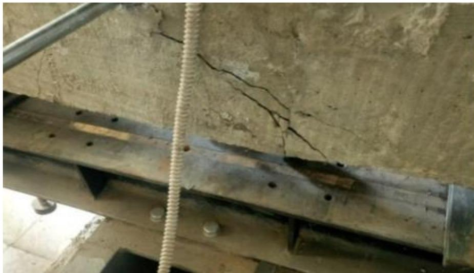
**Figure 19:** Failure of Quarter flexural beam (FB-V1/4) specimen.
