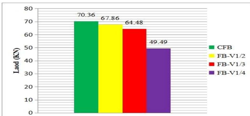
**Figure 21:** Load variations for flexural beam specimens.
