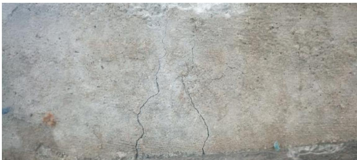
**Figure 18:** Flexural cracks for control flexural beam (CFB) specimen.
