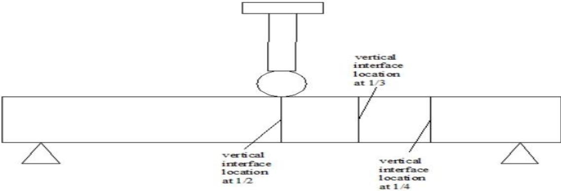
Figure7: vertical interface locations for flexure critical beam.
