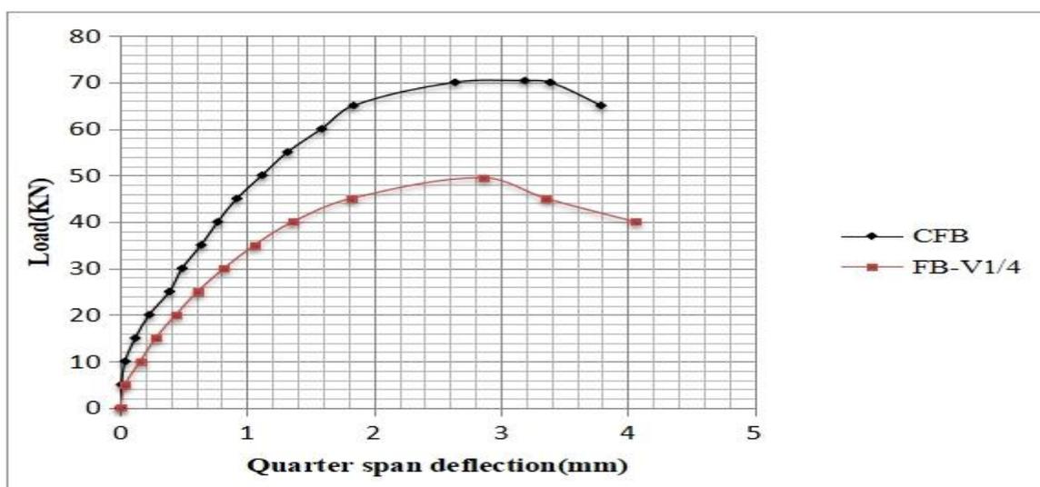
**Figure 23:** Relative load-deflection curves for flexural beams (CFB vs FB-V1/4).
