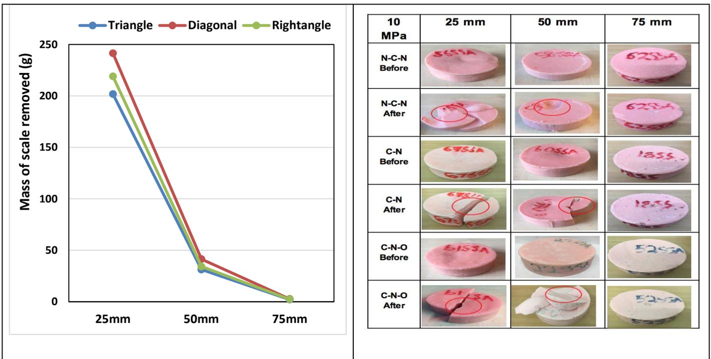
**Figure 14:** Descaling results of solid shaped paraffin scale deposits in the compressed chamber condition
