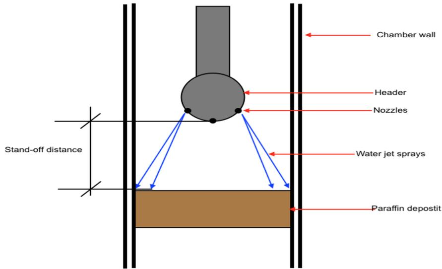
Figure 4: Stand-off distance for solid and hollow paraffin.
