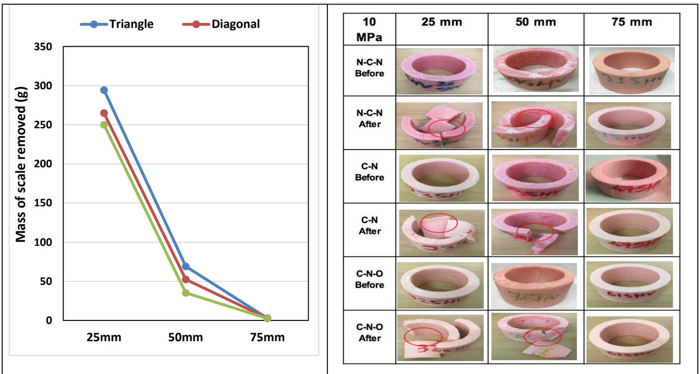
**Figure 12:** Descaling results of hollow shaped paraffin scale deposits in the vacuumed chamber condition
