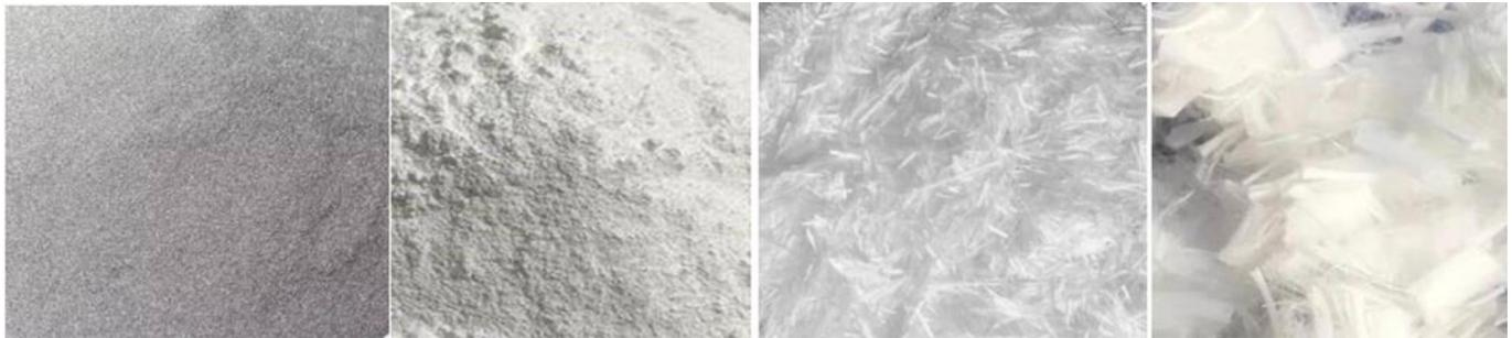
**Figure 1:** Examples of materials utilised for reinforcing PMMA. From left to right: titanium dioxide nanoparticles, alumina nanoparticles, glass fibers, polyester fibers.
