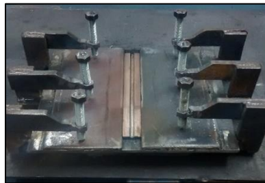
Figure 2: Fixing and backing device for the joint root support.
