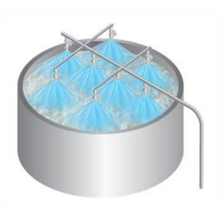
Figure 2: Foam Control by Spray nozzles [16]
