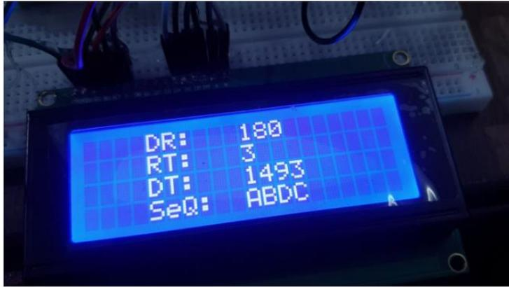
**Figure 8:** LCD showing the inputted parameters value and sequence while operating
