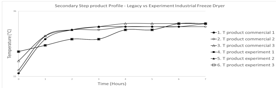
Figure 6: Comparison secondary drying product profile commercial (legacy) vs experiment.
