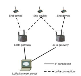
Figure 2: LoRaWAN Network Architecture
