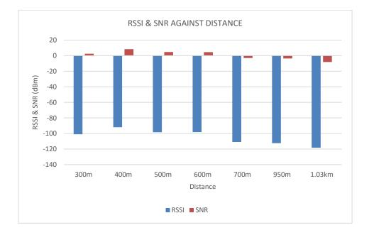
Figure 6: Plot showing RSSI at different distances
