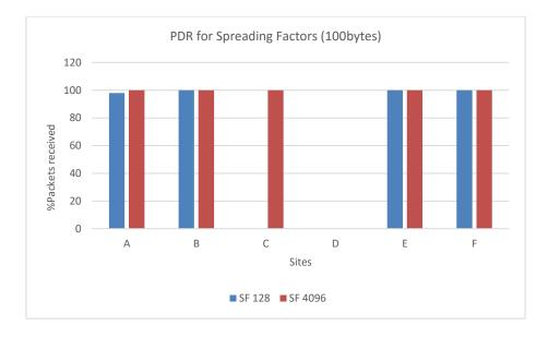
Figure 8: PDR for SF=128 and SF=4096 with payload size 0f 100bytes
