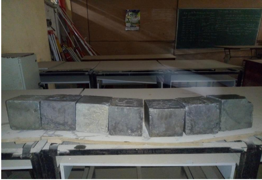
Plate 2: Demoulded Cubes Ready for Curing
