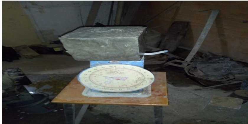
Plate 5: Weighing the Sandcrete blocks before Crushing
