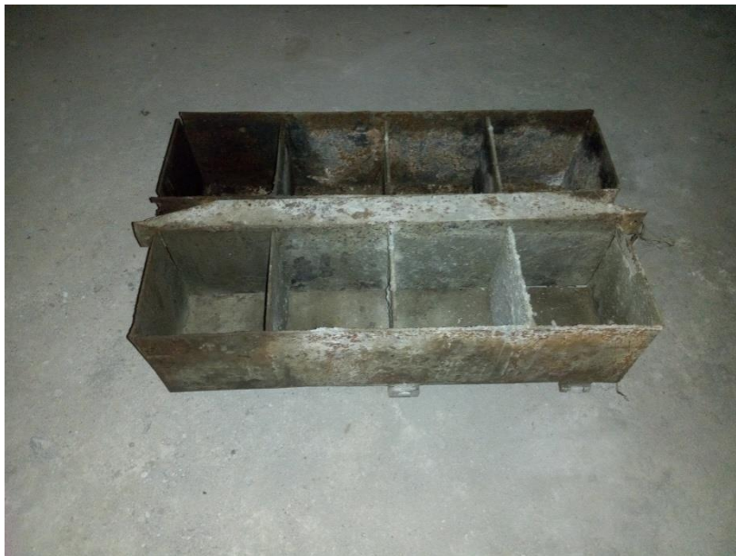
Plate 1: Moulds for Casting Cubes
