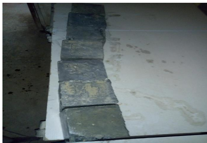
Plate 4: Blended Sandcrete blocks at Different Replacement Levels after Curing ready for Crushing
