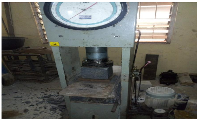
Plate 6: Crushing the sandcrete blocks for Compressive Strength Measurement
