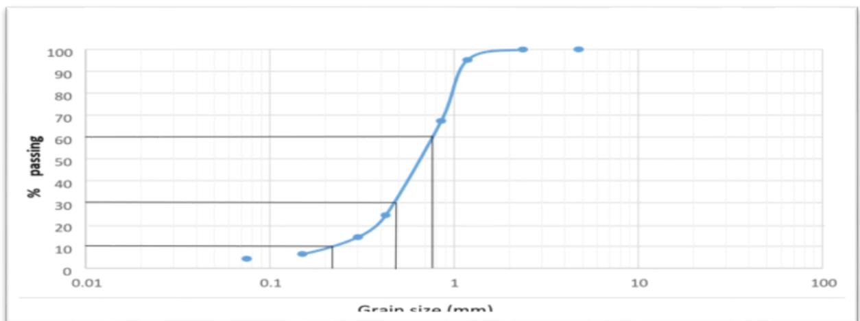
**Figure 3:** Particle soil distribution of bare soil sample (1)
