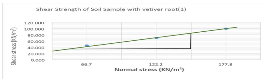
**Figure 6:** Shear strength graph of soil matrix with Vetiver roots (1)
