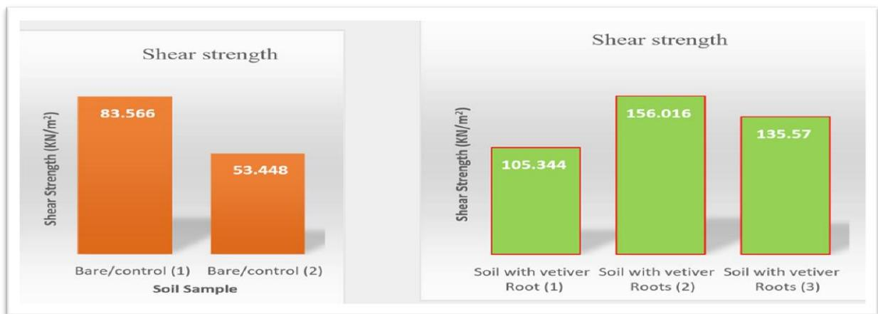
**Figure 10:** Comparison of shear strength result between bare soil and Vetiver grassed soils
