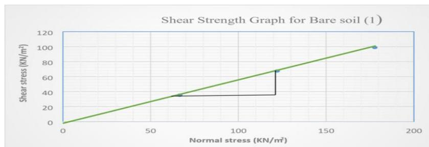
**Figure 5: Shear strength graph of bare soil sample (1)**
