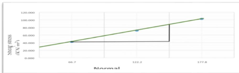
**Figure 7:** Shear strength graph of soil matrix with Vetiver roots (2)
