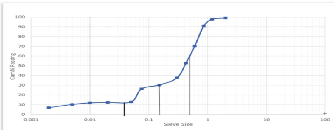
**Figure 4:** Particle soil distribution of bare soil sample (2)
