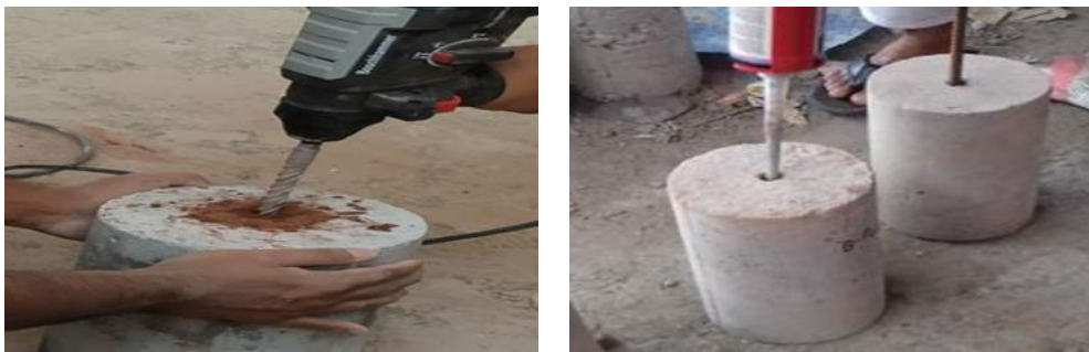
Figure 3: Drilling operation and injecting adhesives operation
