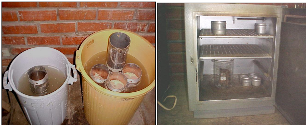
Figure 3: Laboratory analysis. (A) Soil saturation through the process of communicating vessels. (B) After completely drained, the sample is placed in the oven.
