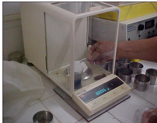
Figure 1: Data collection procedures: (A) Weighing the filter paper on an analytical balance using tweezers (B) Filter paper placed for drying in an oven at 105°C to obtain moisture (C) Weighing the ring + ground.
