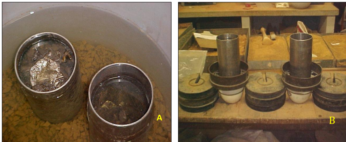
Figure 5: Procedures in the laboratory (A) Sample saturation by the process of communicating vessels (B) Free Drainage of the Waste sample.
