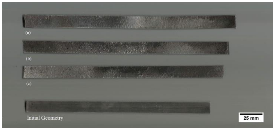
Figure 5: Final geometry of specimens after hot rolling process. Height reductions of (a) 21%, (b) 17% and (c) 13%.
