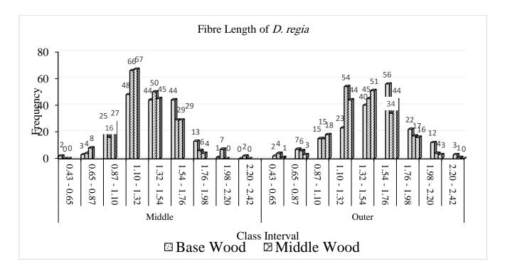
Figure 2: Histogram chart of *D. regia* Fibre length distribution for Middle and Outerwood samples
