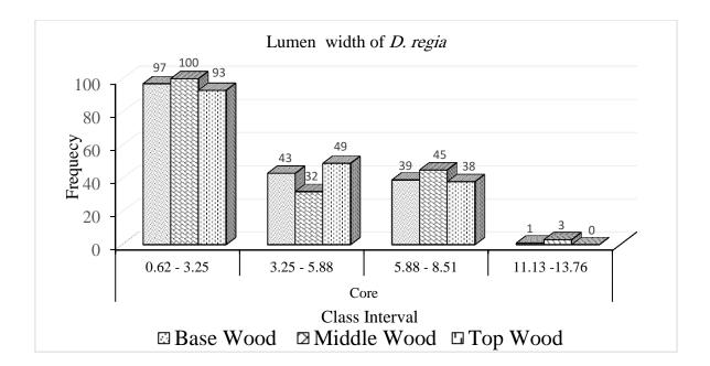
Figure 5: Histogram chart of D. regia Lumen width distribution for Corewood samples
