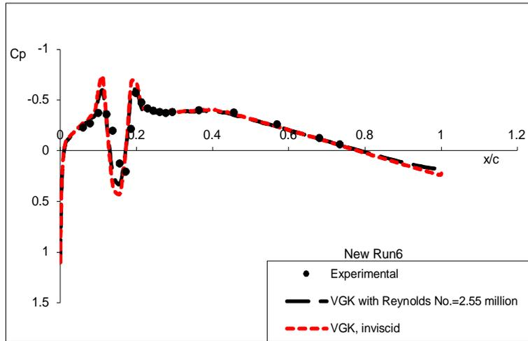
**Figure 10:** Experimental data compared with VGK theoretical predictions using (I0081020) profile.  $M_\infty=0.6123$ ,  $\alpha=0.0$  degrees. Sampling frequency=25 Hz with 10 samples at each port
