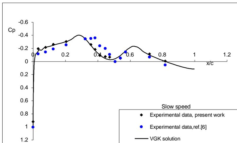
**Figure 8:** Slow speed experimental and theoretical (VGK) upper surface Pressure distribution, (for I0072468, measured geometry used in VGK)
