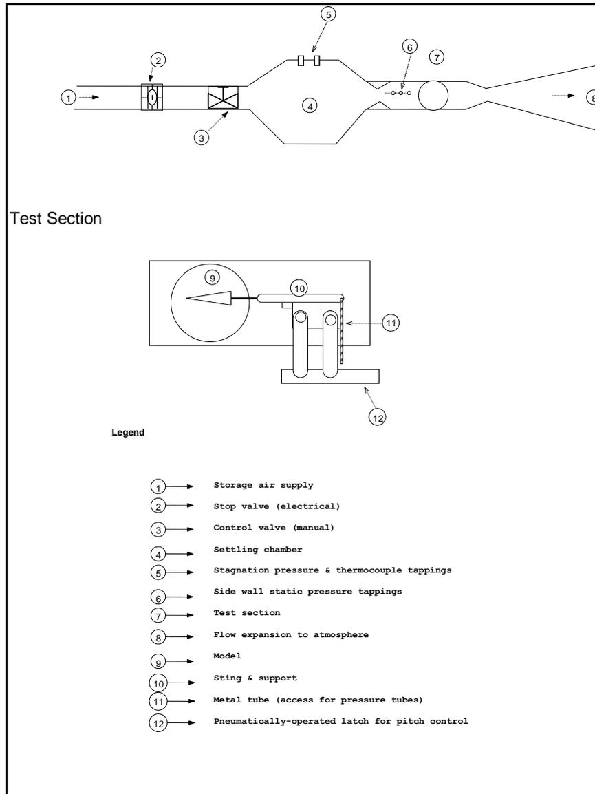
**Figure 1:** Supersonic wind tunnel schematic diagram
