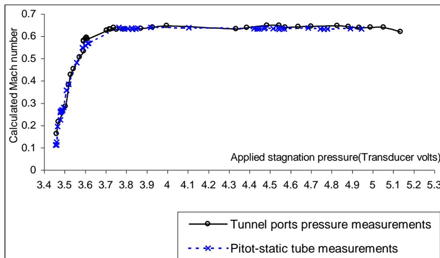
Figure 2: Tunnel Calibration
