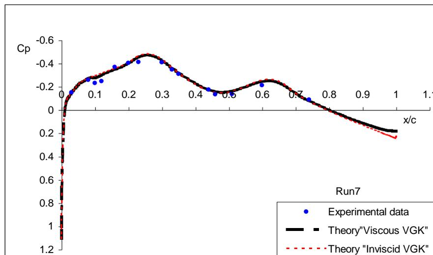
**Figure 9:** Experimental data compared with VGK theoretical predictions using (I0082070) profile.  $M_\infty=0.613$ ,  $\alpha=0.0$  degrees. Sampling frequency=12 Hz with 10 samples at each port
