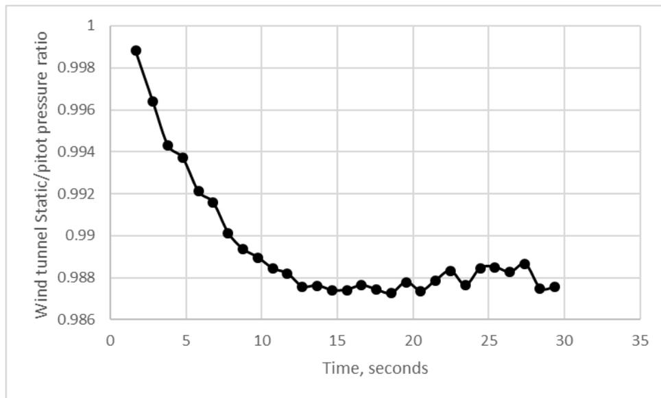
**Figure 11:** Variation of tunnel static pressure with applied pitot pressure (Sampling rate at 12 Hz), standard deviation for the whole run time =0.2905%, standard deviation for data after 15 seconds (settling time) = 0.045%
