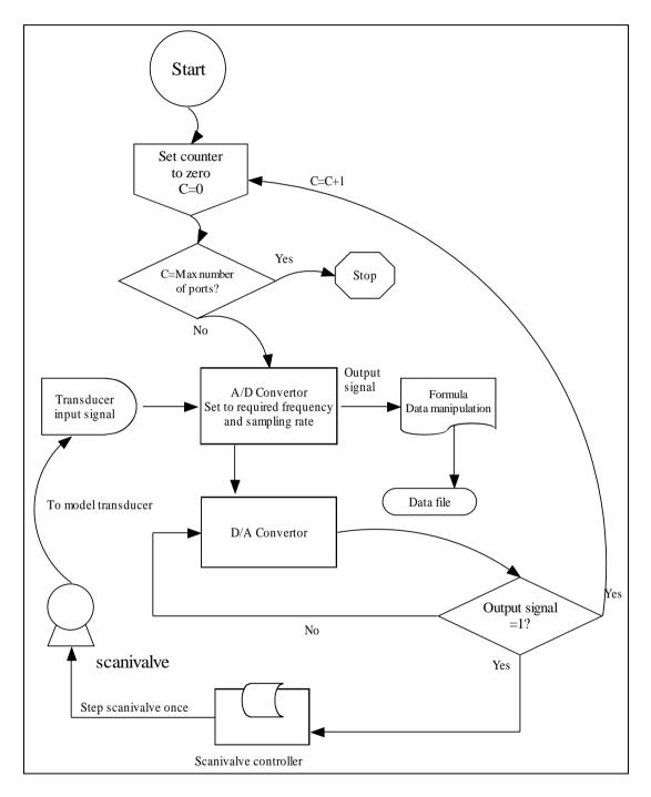
Figure 6: Data acquisition programme "scan data.vee" flow chart
