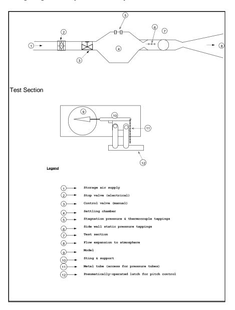
Figure 1: Supersonic wind tunnel schematic diagram
