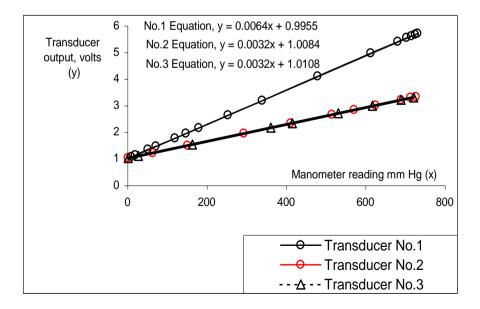
Figure 5: Transducer calibration results
