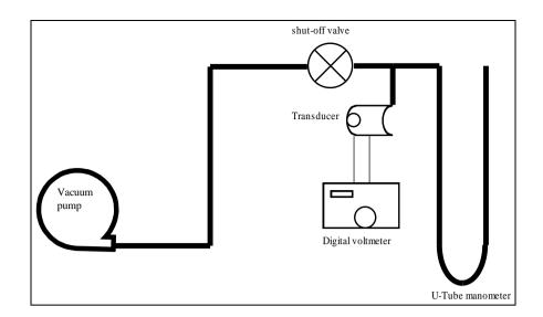
Figure 4: Transducer calibration set-up
