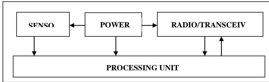
**Figure 1:** Basic architecture of a sensor node.
