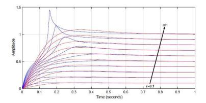
Figure 12: Step responses of the nonlinear system (blue) and multimodel(red) corrected by the CRONE controller.
