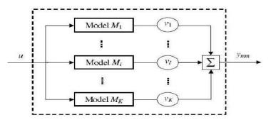
Figure 2: Fusion Principle
