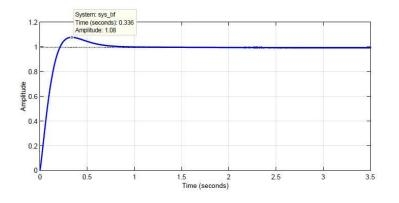
Figure 3: Step response of the model 1
