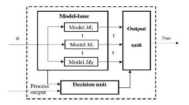
Figure 1: Multimode Approach Principle
