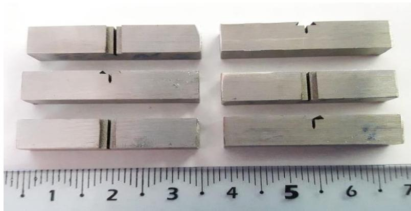
**Figure 2:** SE (B) test-ready specimens.
