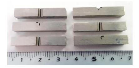
Figure 2: SE (B) test-ready specimens.
