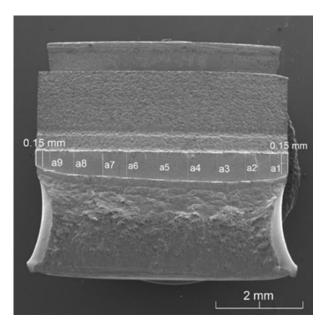
Figure 4: Detailing for crack measurement (60x magnification).
