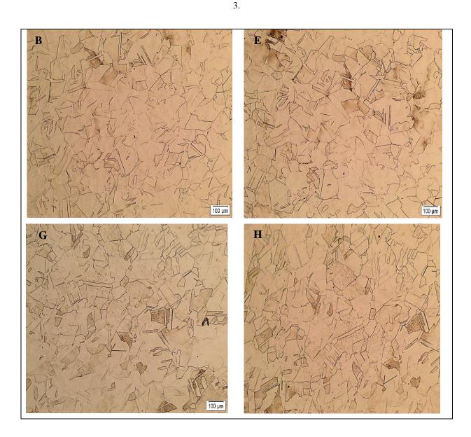
The micrograph observed in the collected samples resembles those found in reference bibliographies and presents the same morphology, making it possible to easily identify it as stainless steel with austenitic structure, with presence of maclas and equiaxial grains, which is compatible with the standards [3]. After, grain size measurements were performed, from these evaluations the software automatically generates reports with the average size calculations and their standard deviations (table 3).
