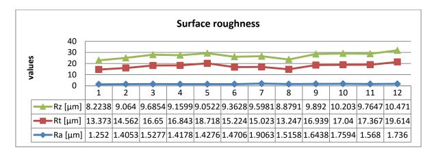
Figure 2: Measured value of surface roughness.
