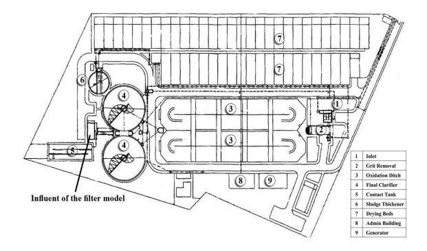
Figure 1: Layout of Saft-Trab WWTP
