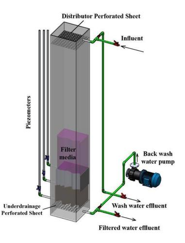
Figure 2: The experimental model of the filter
