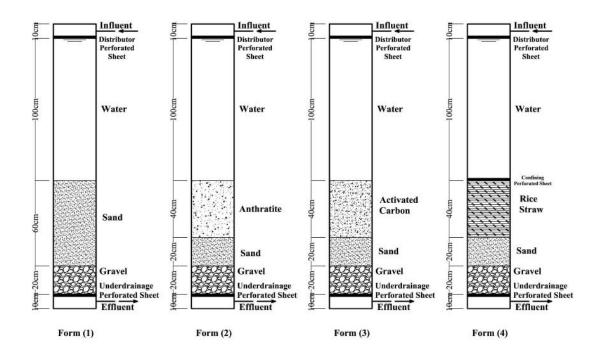
Figure 3: The different arrangements of filter media
