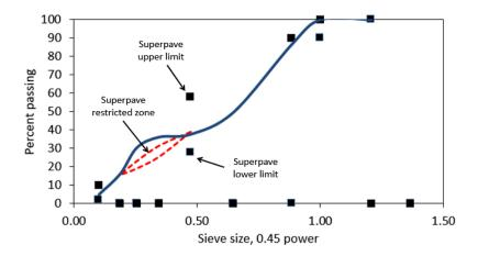
**Figure 4:** Aggregate gradation.
