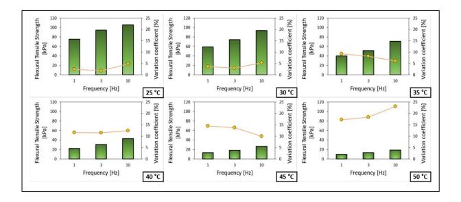
**Figure 5:** Flexural tensile strength, in kilopascals (kPa), registered in 4PB mechanical tests and corresponding statistic variation coefficient.
