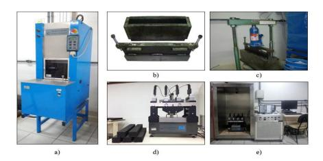
**Figure 3:** a) Superpave Gyratory Compactor (GEOTEC/UFAM). b) Molding apparatus [22]. c) Compaction system [22]. d) *IPC Global* Four-Point Bending apparatus. e) Data acquisition system, including climatic chamber and *IPC Global* 4PB equipment [22].
