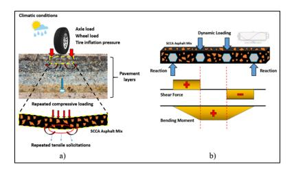
**Figure 1:** a) Scheme of asphalt coating layer deformation, submitted to climatic and traffic solicitations. b) Four-point bending test beam model and characteristics shear force and bending moment diagrams.
