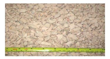
Figure 2: Sinterized Calcined Clay Aggregate (SCCA) after controlled calcination and crushing process.
