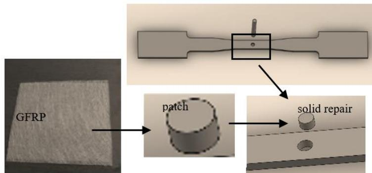
**Figure 2:** Solid repair of damage model composite
