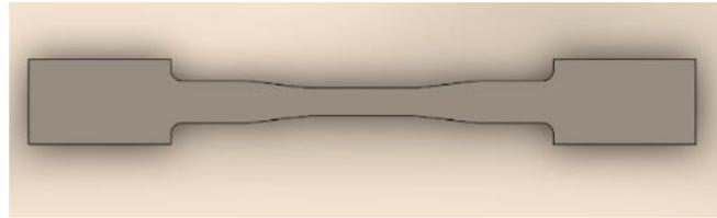
a. Tensile test specimens of GFRP
