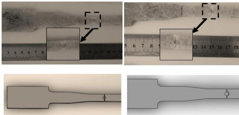
**Figure 5:** Macrographics of Fracture at Repaired Composites Tensile Tested
