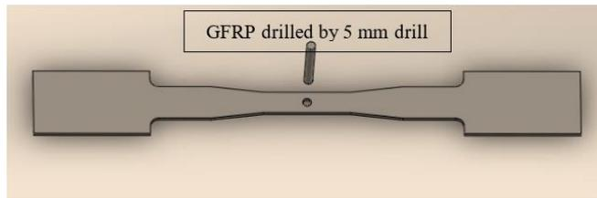
b. Modeled damaged composite (HGFRP)
