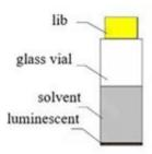
Figure 5: Liquid Scintilation detector
