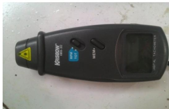
**Figure 6:** Tachometer
