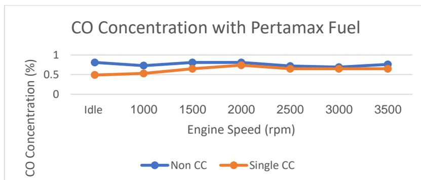
**Figure 8:** CO concentration on pertamax fuel with variations in engine speed
