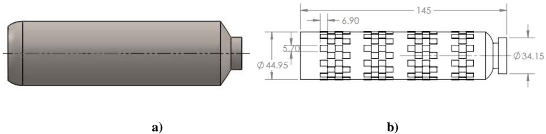
**Figure 4:** (a) casing of catalytic converter (b) dimension of catalytic converter core
