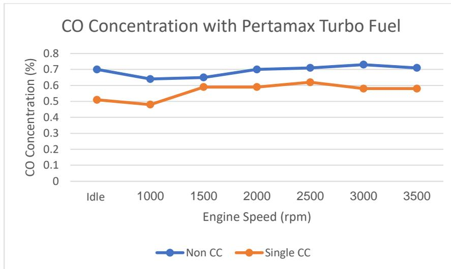
**Figure 9:** CO concentration in the pertamax turbo fuel with variations in engine speed
