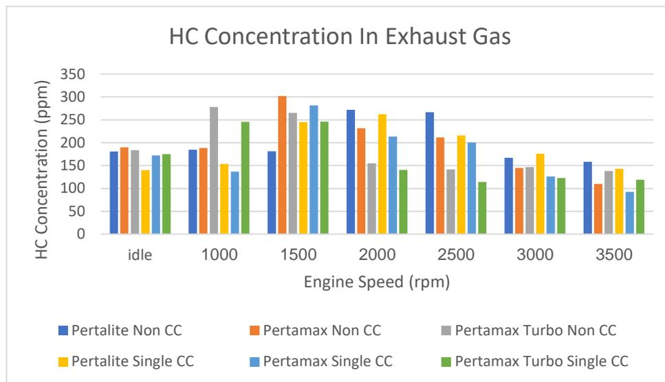
Figure 14: HC concentration in 3 types of fuel
