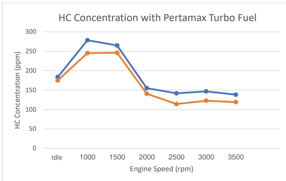
Figure 12: HC concentration in pertamax turbo fuel with variations in engine speed
