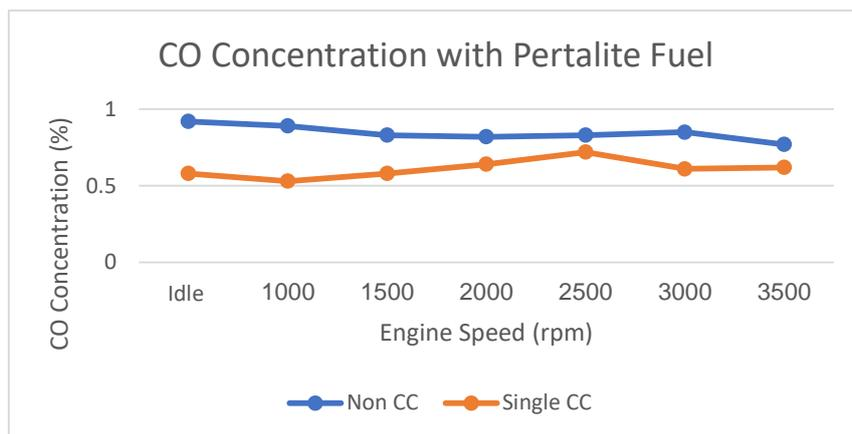
**Figure 7:** CO concentration in pentalite fuel with variations in engine speed
