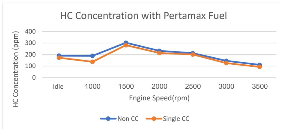
Figure 11: HC concentration in pertamax fuel with variations in engine speed
