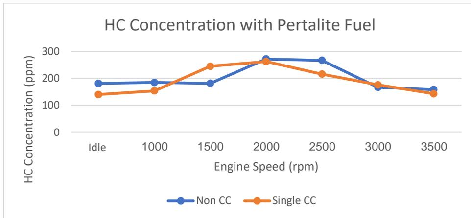
Figure 10: HC concentration in peralite fuel with variations in engine speed
