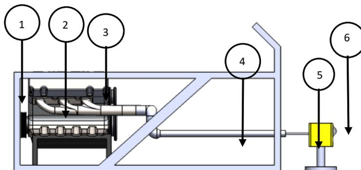
Figure 2 (a): Set up equipment without catalytic converter
