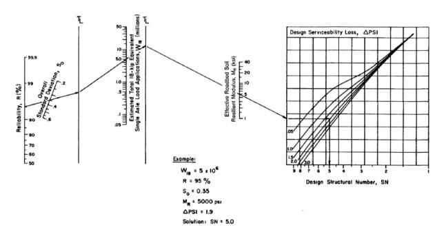
Figure 3: AASTHO Flexible Pavement Design Nomograph [15]
