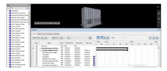
Figure 5: Showing the selection set and timeliner for simulation
