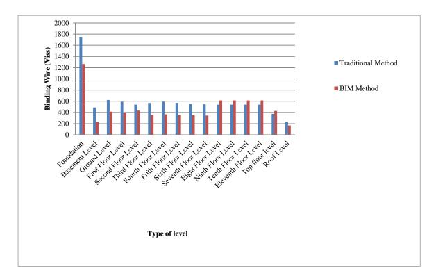
Figure 17: Quantities of Binding Wire in each level
