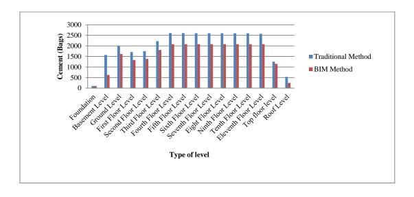
Figure 12: Quantities of cement in each level
