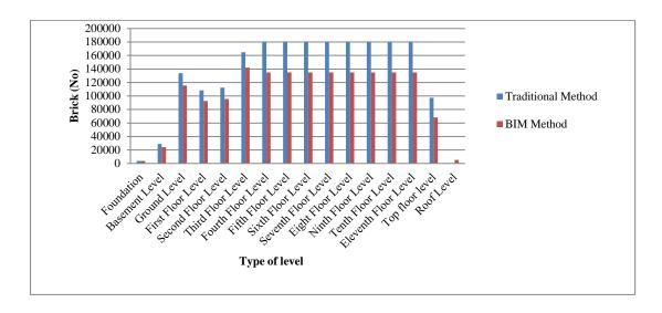
Figure 15: Quantities of brick in each level
