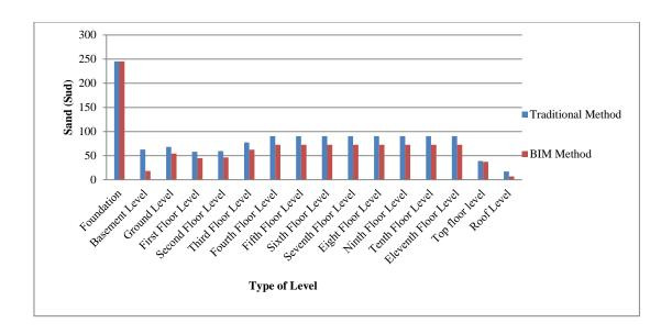
Figure 13: Quantities of sand in each level
