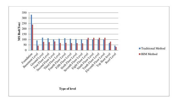
Figure 16: Quantities of MS Rod in each level
