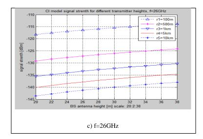
Figure 2: Plot showing received signal strength against BS antenna height for the various distances
