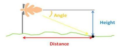
Figure 3: Relationship between antenna height, tilt and T-R distance
