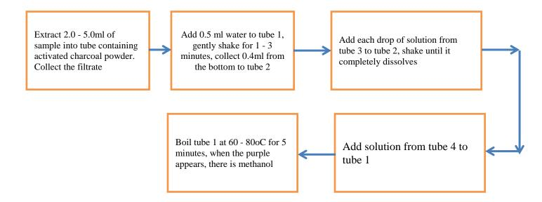
Figure 9: Unauthorized methanol discovery process in gasoline.
