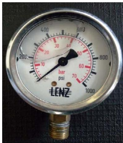
**Figure 1: Bourdon Pressure Gauge**
