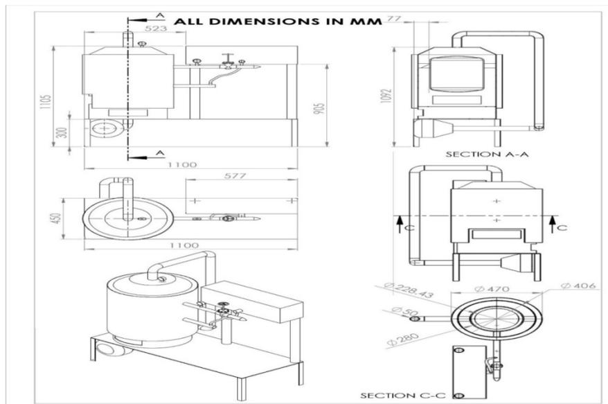
**Figure 4:** The two-dimensional view of the boiler
