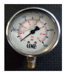
Figure 1: Bourdon Pressure Gauge
