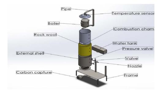
Figure 5: Exploded View the boiler
