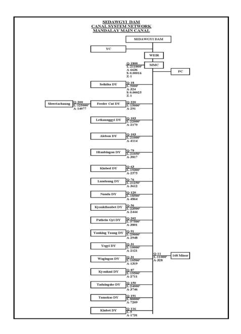
Figure 2: Canal Network System of Mandalay Main Canal in Saedawgyi Irrigated Area
