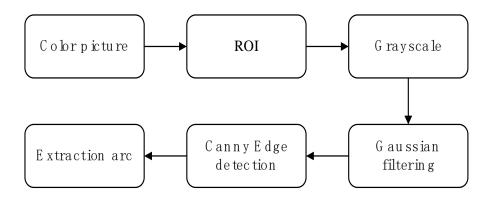
Figure 1: Extract arc processing
