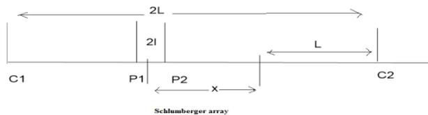
$$\rho_a \approx \rho_1 \left[ 1 + 2 \sum_{m=1}^{\infty} \left[ \frac{k^m}{\{1 + (2mz/L)^2\}^{3/2}} \right] \right] \dots \dots \dots (1)$$
