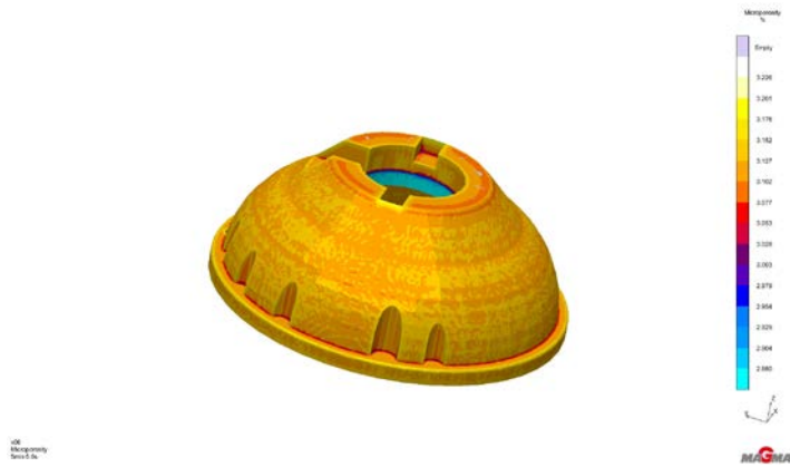
Figure 6: Microporosity Result on Cold Mould
