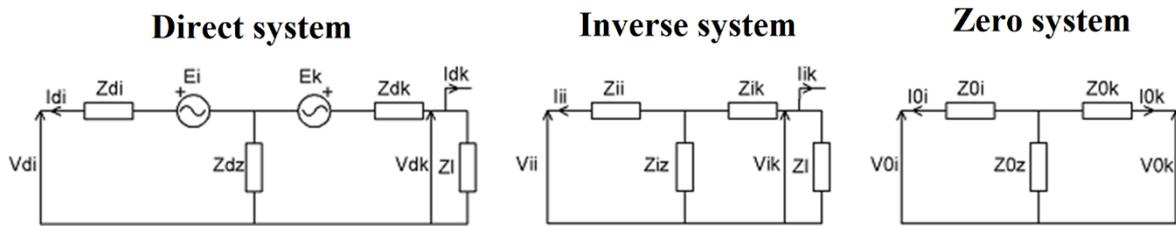
Figure 3: Equivalent scheme for the calculation of cross-country fault
