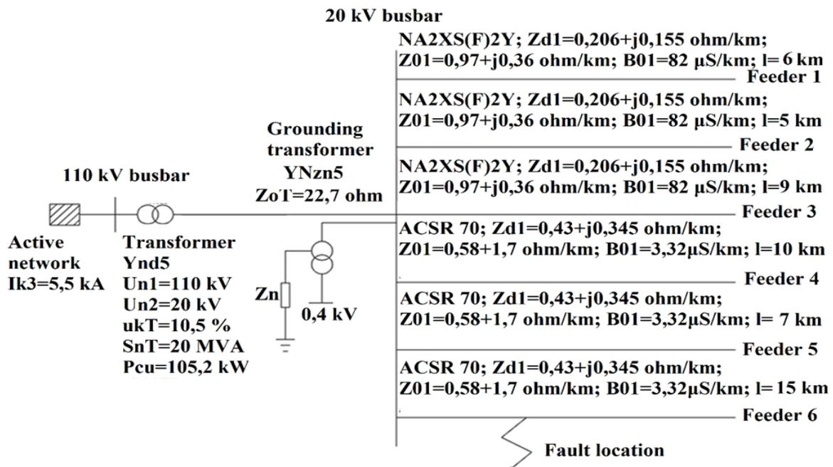
**Figure 4:** Case study 20 kV distribution network
