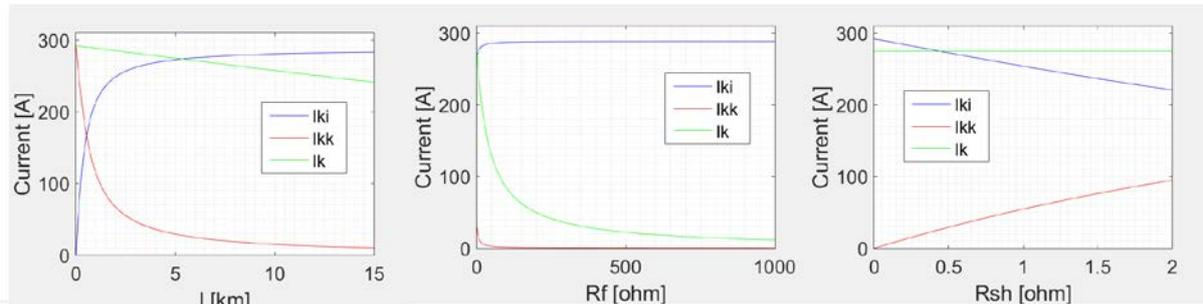
Figure 7: Dependences of the fault currents model without load - high-resistance network earthing
