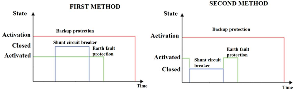
**Figure 2:** Coordination between the shunt circuit breaker operation and definite-time earth fault protection
