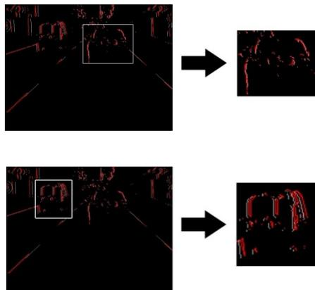
**Figure 4:** (left) Edges detection satisfied formula (1). (Right) bounding box detection
