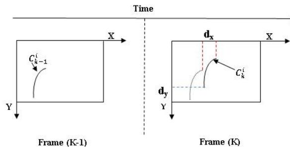
**Figure 2:**  $I_{k-1}$  and  $I_k$  represent the displacement value of the edges  $C_{k-1}^i$  in the scene  $S_k$ .
