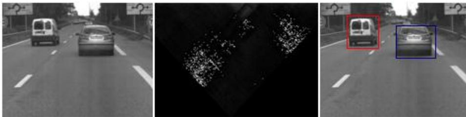
**Figure 5:** Symmetry detection; (left) initial image. (Center) symmetry map, (right) vehicle detection.
