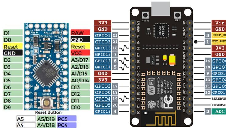
Figure 1: Pin structures of NodeMCU and Arduino Pro Mini.
