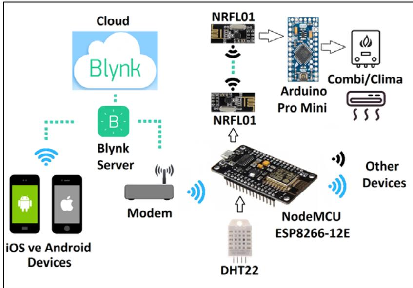
Figure 4: Structure of the System
