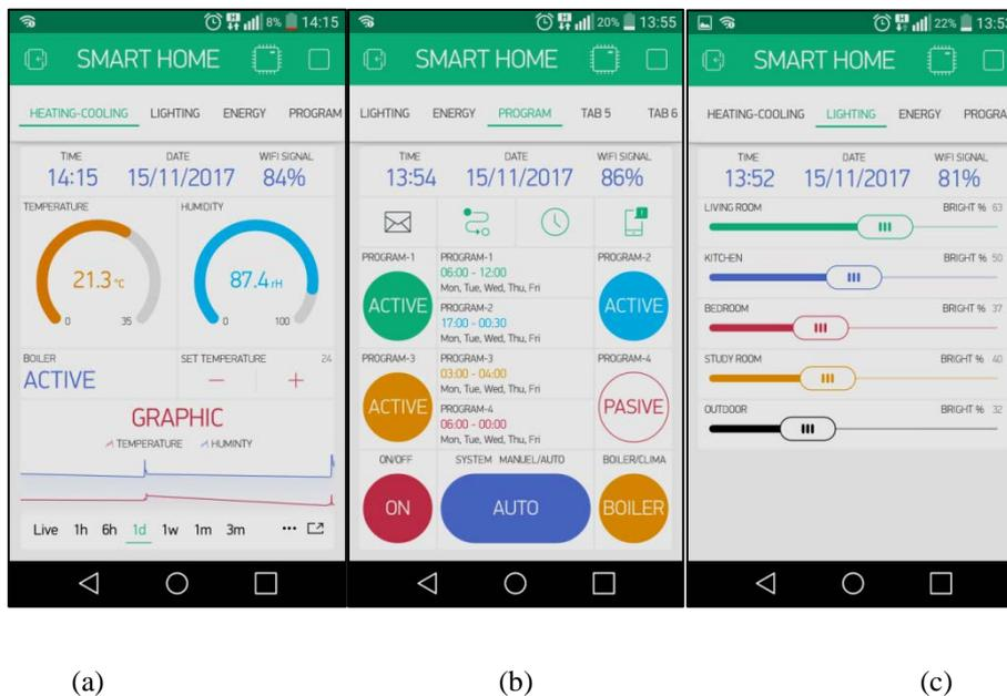
Figure 5: Blynk "SMART HOME" user interfaces a) air conditioning b) weekly schedule c) lighting
