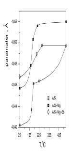
Figure 1: Change of latice parameter of Al matrix after isothermal annealing
