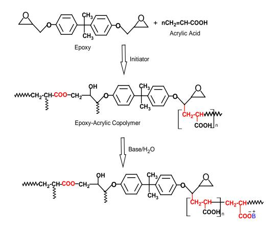
Figure 6: Acrylic acid grafted waterborne epoxy
