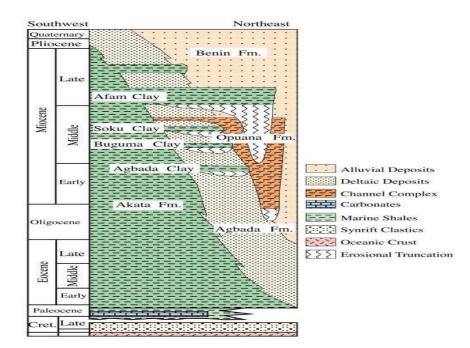
Figure 4: Stratigraphic framework of the Niger Delta modified from [2]
