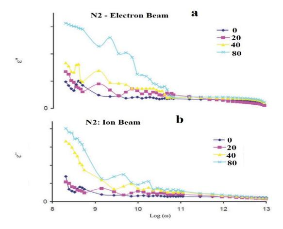
Figure 8: Variation of the imaginary part of the impedance  $\varepsilon$ " with frequency for film at room temperature, irradiated and non-irradiated with electron and ion beams
