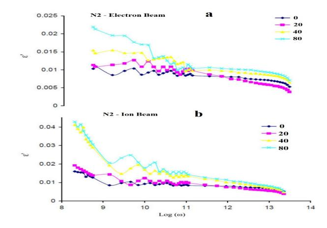
Figure 7: Variation of dielectric of film for all irradiated and non-irradiated samples with electron and ion beams at room temperature
