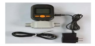
Figure 2: Digital Gas meter, model MF5706-N-200
