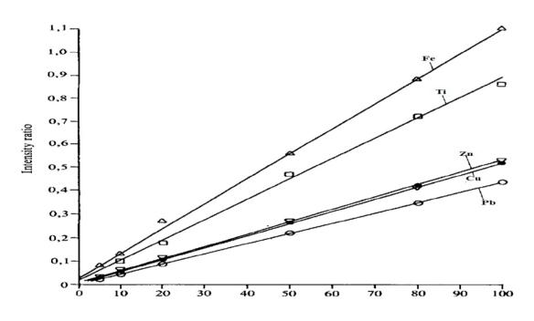
Figure 11: Calibration for the determination of lead, iron, copper, titanium and zinc by the Coprecipitation method
