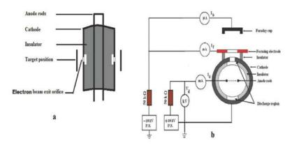
Figure 5: Schematic of the double beam source, a. Electron source and b Ion source [16]
