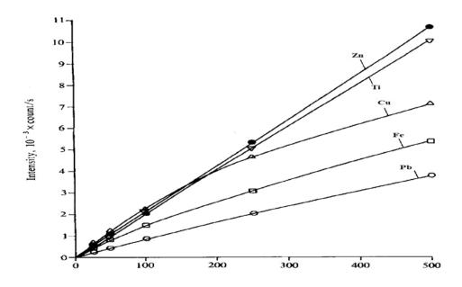
Figure 10: Calibration for the determination of lead, iron, copper and zinc by the direct filter- paper method.
