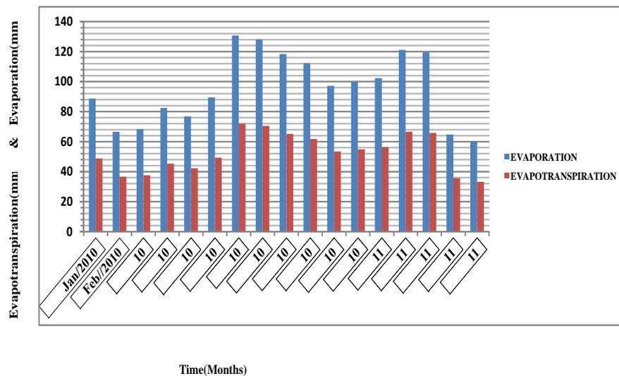
**Figure 4:** Evaporation-evapo-transpiration variability in the Migina (Rwasave evaporation pan)
