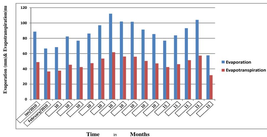
**Figure 5:** Evaporation-evapo-transpiration variability in Migina (Gisunzu-evaporation pan).
