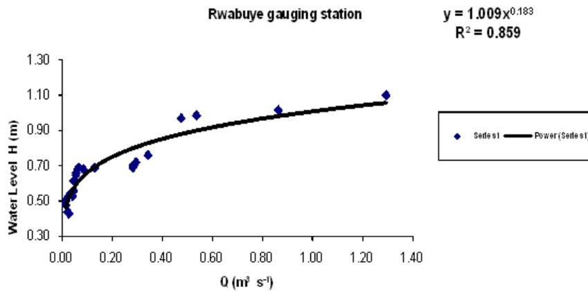
**Figure 6:** Water Level Vs Discharge at Munyazi-Rwabuye gauging station
